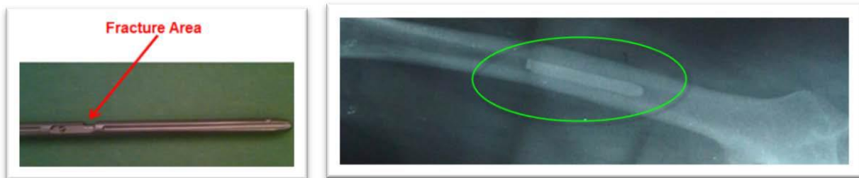
Figure 2: Image of SP2 IM Rod highlighting area of potential fracture / Image of SP2 IM Rod fragment in a radiograph
